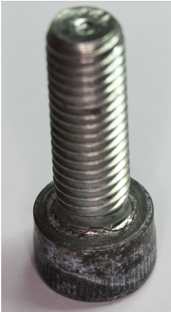
Figure 1 Hydrogen embrittlement of M10 zinc plated SHCS
