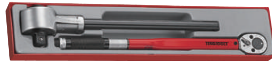
Torque wrench 1/2" drive angular gauge covering 40 to 210Nm (1292AG-EP) Torque multiplier 1/2" F:3/4" M torque multiplier (3 to 1 ratio) and maximum torque capacity 1,500Nm (MP1400)
