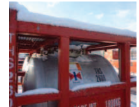
Remove snow, ice or other debris as it adds weight, creates dropped object hazards and obscures other loose items.
