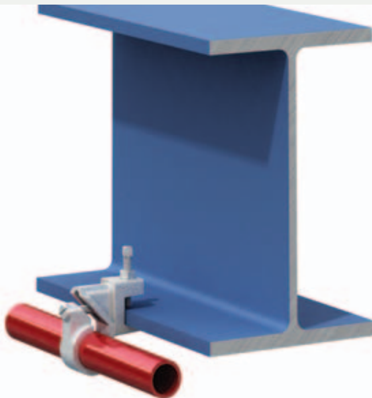
Beam clamp with tapped holes in position X and Y to accept threaded rod or cable clips. For parallel or tapered flanges. Supplied with grade 8.8 cup point setscrew.
