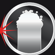
Tungsten Carbide Powder Deposited Through a High Powered Laser to the Blade Edge
